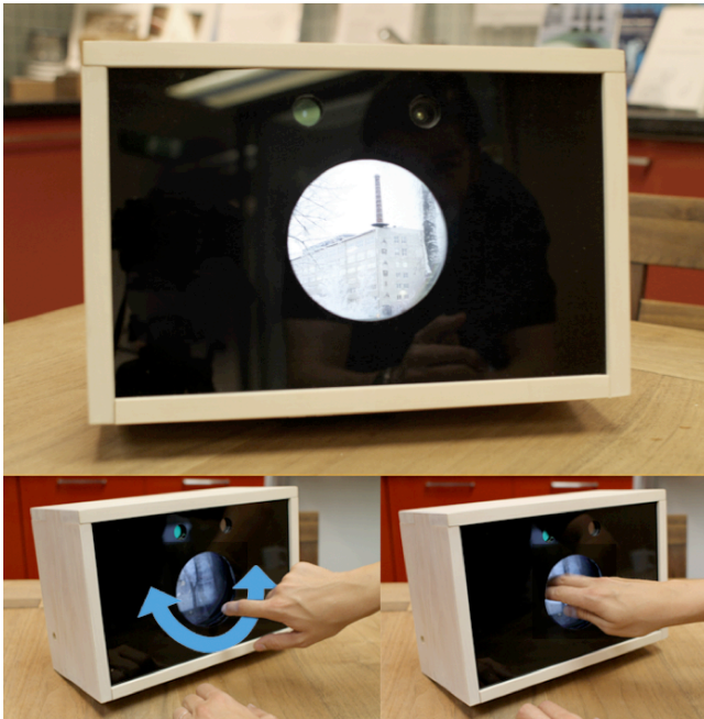
Figure 5. Hole in Space prototype and the tangible interactions enabled by the device.
