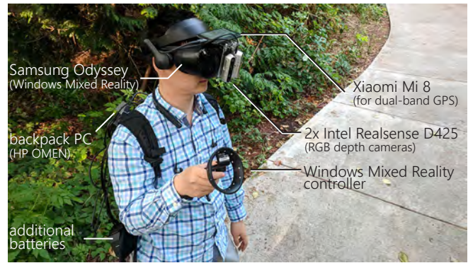
Figure 3. DreamWalker’s mobile virtual reality system, including sensors, computing platform, and display device.
