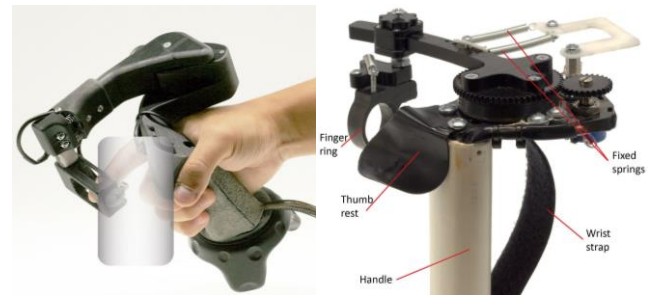
Figure 10: Left) Claw device. Right) Fixed-Spring device. The Spring device was built as a copycat of the other two prototypes CapstanCrunch and CLAW with the difference that the finger arm was only connected to a fixed spring.
