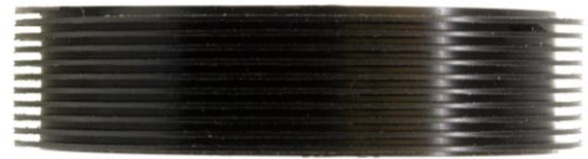
Figure 5: A helix groove machined into the acetal drum to prevent cord overlap.
