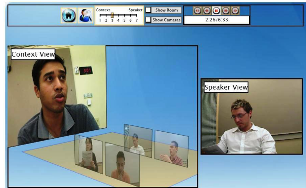
Figure 6. 3D interface in the user-controlled mode configured to show a larger context view.
