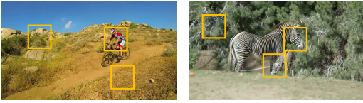
Figure 5: Examples of targets on keyframes. The size of a target equals the receptive field of the input feature map of the scheduler. As shown, a target patch might be an object, a part of an object, or totally background. The “tracking” results of these targets will be fused later. It should be noted that targets include all possible patches in a sliding window manner, but not just the three boxes shown above.
