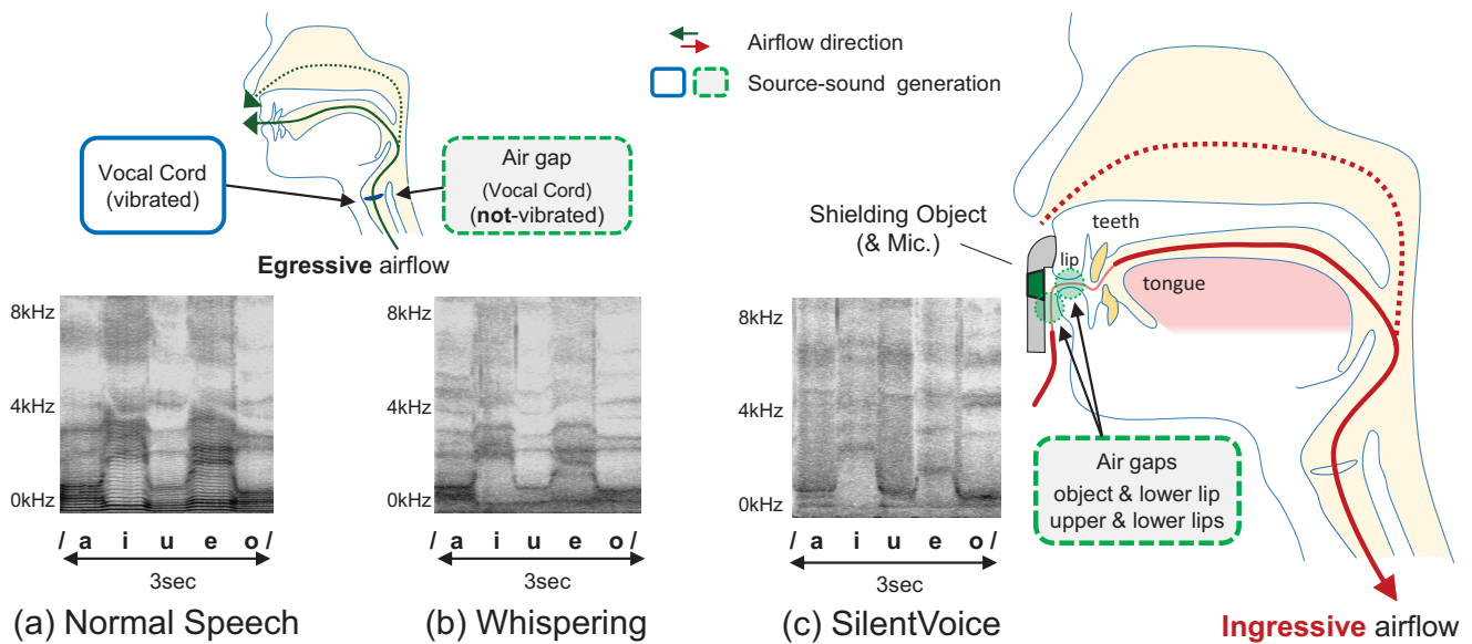
Figure 1: Structure of utterances with spectrograms (/aiueo/): (a) normal speech, (b) whispering, (c) SilentVoice
