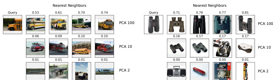
Fig. 1: A pair of sample queries from the Caltech-256 dataset, showing the four nearest neighbors in three different feature spaces. Each neighbor is annotated with its Euclidean distance to the query in that space.
