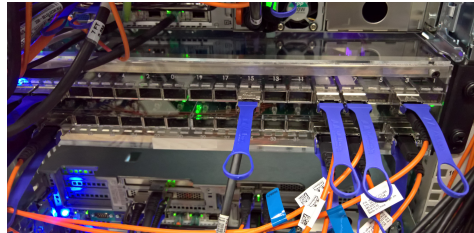
Figure 4: Prototype circuit switch.
