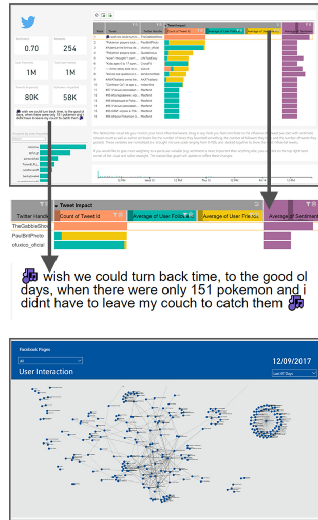
Figure 3. Top: Page from Twitter solution template showing Table Sorter ranking tweets based on the combination of retweets, user followers and friends. The top tweet is selected. Bottom: Page from Facebook solution template showing Network Navigator of users co-posting in the last 7 days.
