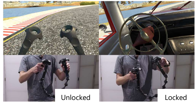
Figure 9. Summoning a vehicle using gestural input (left), then driving with a rigid steering wheel (right).
