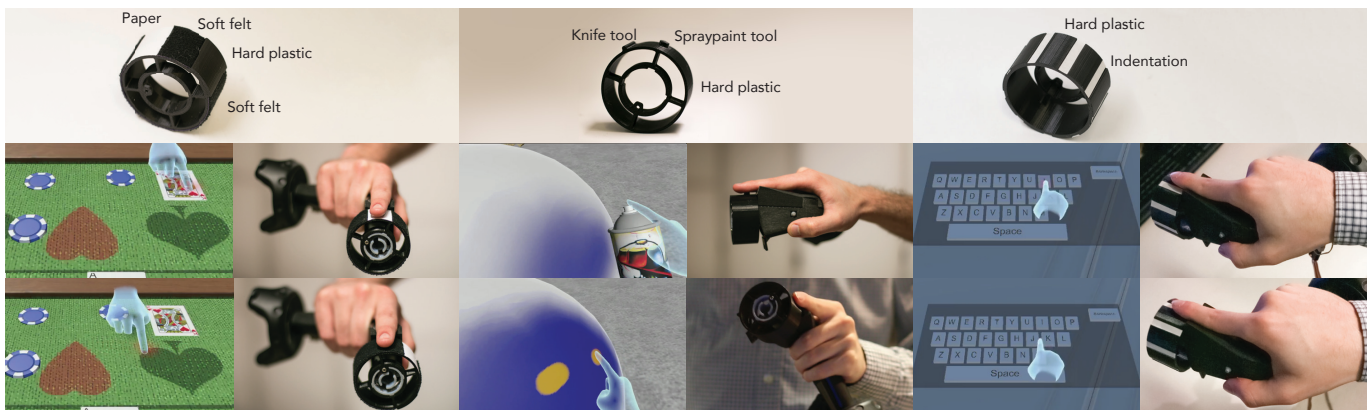
Figure 12. (left) A card table demo that highlights our ability to render different textures. The wheel used in this demo consists of two regions of soft felt, a hard plastic ridge, and a small section of paper. When the user touches an object in the scene, the appropriate texture is placed underneath the fingertip. (center) A painting and sculpting demo that highlights the ability to render shapes and sense the force applied to the wheel. The wheel used in this demo consists of a raised nub and a ridge to simulate holding tools. The user presses on the wheel to activate the tool. The model can be explored by touch. (right) A keyboard demo that highlights our ability to render edges and shapes. The wheel used for this demo consists of nine raised plastic regions with grooves in between. When a user approaches the edge of a key, the edge of a groove is placed under the finger.
