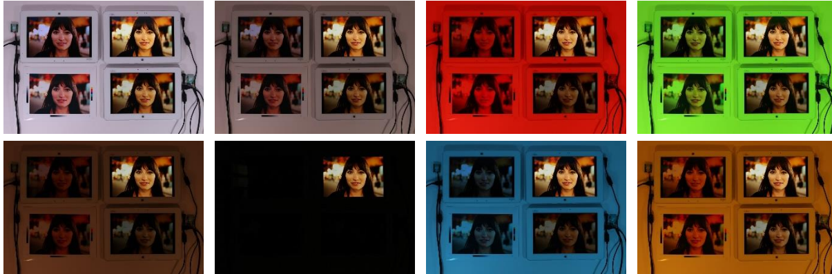
Fig. 1. Eight photos of our test setup, each taken under different colored and brightness ambient lighting conditions. In each photo the calm display (top left) adapts to the lighting in a similar way to paper (bottom left). Common adaptive display brightness (top right) and a calm display without color corrections (bottom right) are shown for comparison.
