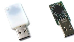
Fig. 3. Custom-built USB dongle with 4-channel (RGB+clear) TCS43275 light sensor.
