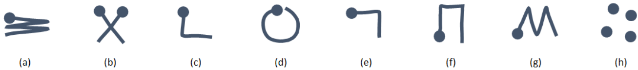
Figure 2. SketchInsight supports eight simple pen gestures. (a)-(b) scribble and ‘X’ for erasure, (c)-(e) ‘L’, ‘O’, and inverted L for X/Y chart, pie chart, and map creation, and (f)-(h) bar shape, jagged line, and four dots for changing a chart type to a bar chart, line chart, and scatterplot.
