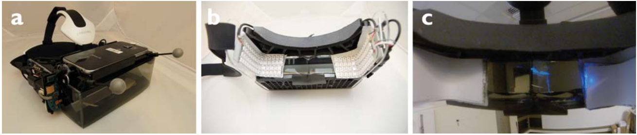
Figure 5. SparseLightAR construction. (a) Our custom AR head-worn display prototype. A Samsung Galaxy S6 is mounted on top, connected to the external IMU and the SparseLightAR controller (left assembly). (b) SparseLightAR LED arrays installed. (c) SparseLightAR with paper diffusers added, in operation showing a scene with flying butterflies (blue).
