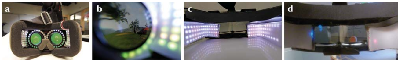
Figure 1. Our sparse peripheral display prototypes: (a) Virtual reality prototype SparseLightVR, with a 170° field of view, showing LED arrangement. (b) SparseLightVR imaged from the inside showing a forest scene. (c) Augmented reality prototype SparseLightAR, with a field of view exceeding 190°. (d) SparseLightAR showing a scene with butterflies and beach balls.
