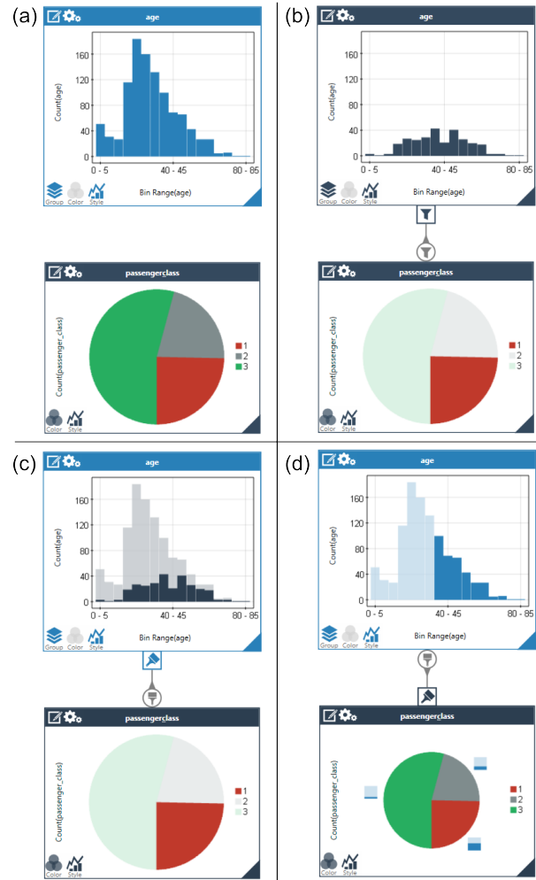
Fig. 5. Four ways to compose two visualizations to show different relationships between attributes. (a) No relationship. (b) Top filters bottom. (c) Bottom brushes top. (d) Top brushes bottom.
