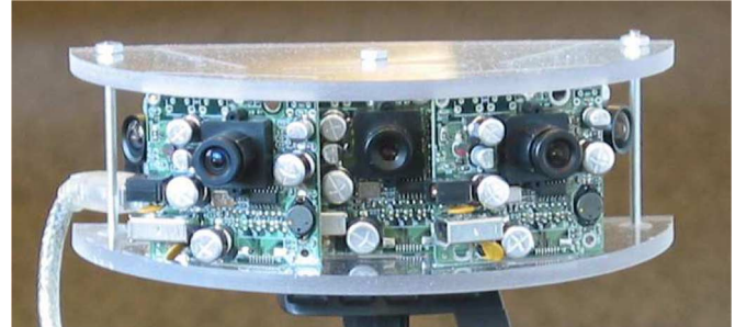
Fig. 5. Half-ring camera which consists of five 1394 fire-wire video cameras. The center camera has the smallest field of view.
