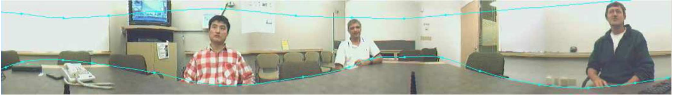
Fig. 7. Two curves on an 360-degree panorama image have different shapes compared with 180-degree images.
