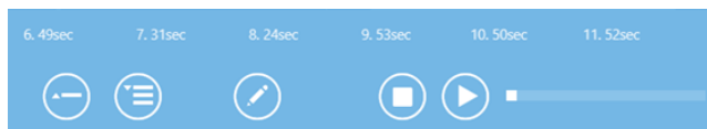
Figure 6. Recording list and media control. A list of annotations, sorted in order of creation, runs across the top. Buttons are used to collapse, expand, edit, stop and play annotations, respectively.
