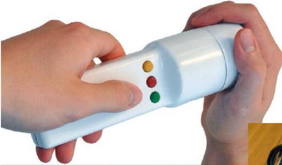
Figure 3. The Peppermill is an interaction-powered user interface device that used to control a TV. Rotating the Peppermill clockwise with the red button p turns up the volume, and with the green button pressed increments the chan
