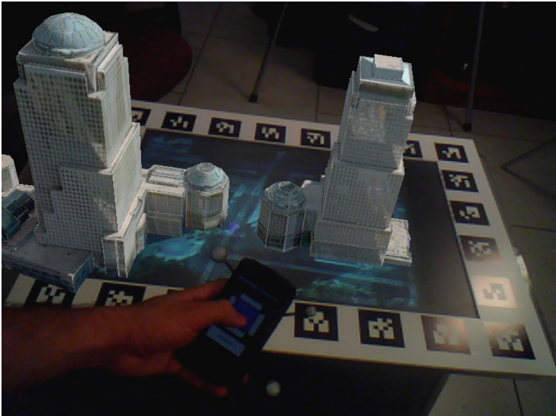
Figure 10. Urban visualization prototype. 3D virtual building models of part of the World Financial Center are presented on head-tracked eyewear and overlaid on the buildings' footprints displayed on Surface using the Bing Maps API. Hand-held smartphone is also tracked relative to the Surface. (Building models courtesy of Bill Chen and Johannes Kopf, Microsoft Research.)
