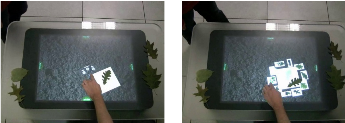
Figure 3. Collaborative multi-user version of the botanical field guide for Surface. (a) User specifies a bounding box for the leaf, places the leaf inside it, and triggers processing by explicitly selecting a user interface element. (b) System captures image of leaf, segments it, displays segmented image in green for feedback, performs matching, and surrounds leaf with images of potential matches.
