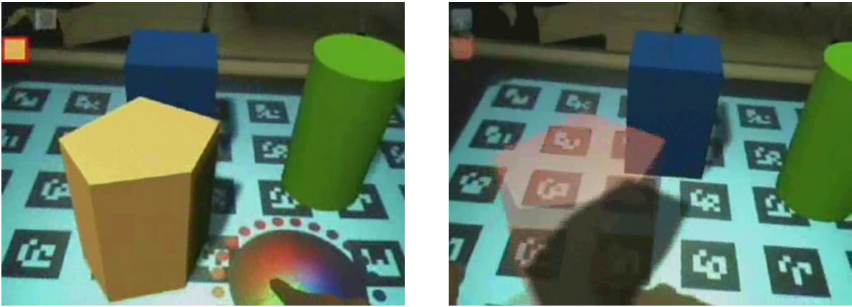
Figure 7 (cont.). Simple CAD prototype using tracked video-see-through eyewear with Surface. (c) Changing the color of an object. (b) Translating an object on the Surface.
