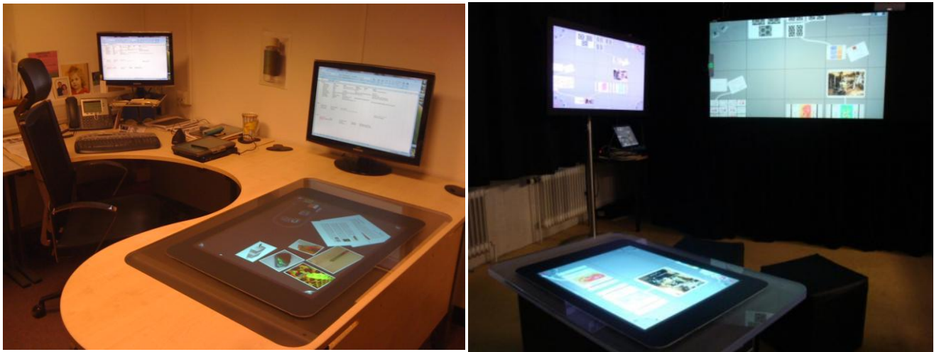
Fig.2: a) Integrated desk installation at NP centre. b) Mediaroom lab facility of the University of Konstanz. The DeskPiles system successfully allows many of the features described in the plan for this project, including on-the-fly annotation, and use of tablet PCs for pen input together with the Surface for multitouch manipulation of the piles.
