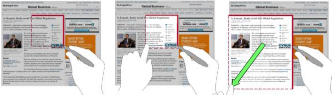
Figure 9. Drawing a crop mark (red polyline from left to right and then down) displays a feedforward selection/clipping marquee widget. Dragging the marquee while drawing switches to bi-manual selection.
