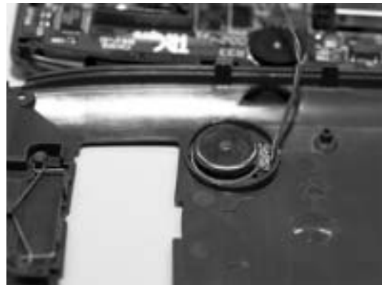
Figure 1: Example of actuator mounting Putting actuator on the back panel of PDA.
